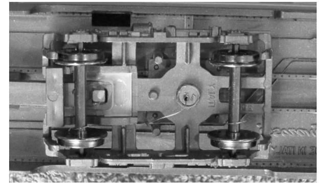
The phosphor bronze wire should be next to the non-insulated side of the wheels. Bend and cut off excess wire from the other end. Insert the magnet wire into the drilled out kingpin hole. Solder the magnet wire to the phosphor bronze wire. Be sure to pre-tin the magnet wire. Sustained heat is needed to burn off the insulation on the magnet wire.
