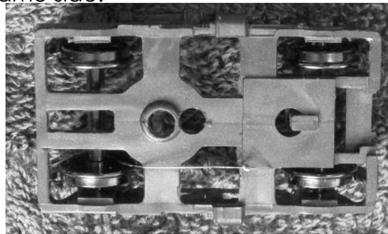
Insert the phosphor bronze wire as shown above. Two kinds of wires are supplied. The phosphor bronze wire is not coiled and is like a spring. Bend a hook in the wire as shown to secure the wire.
